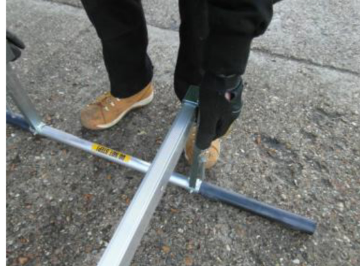
Slide the eaves batten over the stiles of the footing Ladder and locate using the captivated pins into the height adjustment holes of the stiles. Ensure the pins are pressed home fully.
