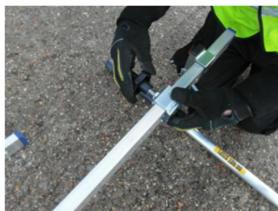
Screw the two Wheel screws into the sliding shoes.
