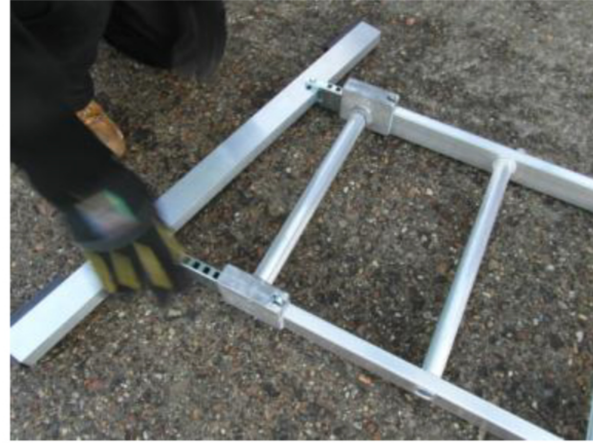
Push the stabiliser foot into the bottom of the footing Ladder.
